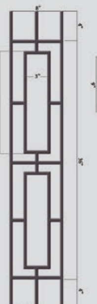
HF 9.4.2 Ends: 1/2" Sq. Height: 44" Wt. 4.8 lbs. TUBULAR (Level)
