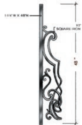
RIGHT TERMINATION LEFT SIDE VIEW
