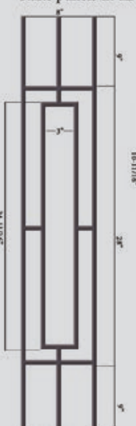
HF 9.4.11 Ends: 1/2" Sq. Height: 46" Wt. 4.5 lbs. TUBULAR (Rake)
