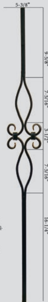
HF 16.8.9 Ends : 5/8" Sq. Height: 44" Wt. 4 lbs. TUBULAR
